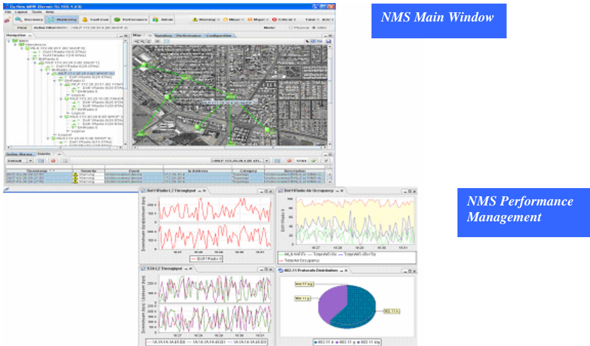
Figure 2 NMS managing a large metro broadband wireless network
